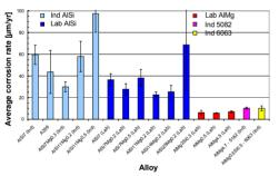
As expected, AlMg(Si) alloys had low corrosion rates in natural sea water. The corrosion rate of AlSi castings were higher. The effect of Si on corrosion susceptibility of AlSi was not clear.
